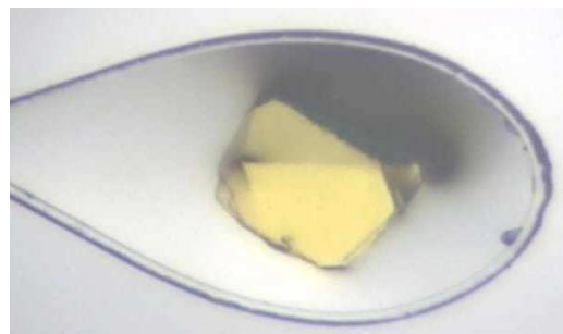
Fig. 3. The protein crystal (measured about 100 \mu\text{m} across) suspended in a tiny loop, prepared for the X-ray diffraction experiment. The loop is used to fish out the crystal from the crystallization drop, and then to place it immediately in a stream of nitrogen gas at 100 \text{ K} . In this way, the water inside and around the crystal is vitrified (i.e., becomes amorphous and does not interfere with the protein diffraction). By the same trick, the crystal is protected from drying and its structure is "stabilized" because with a lowered temperature, the thermal motions of its atoms (expressed by the B -factors) are much reduced. Most importantly, however, the solidified water component of the crystal will drastically slow down the diffusion of free radicals, which are always created on exposure to the ionizing radiation, thus improving the longevity of the crystal. Courtesy of Dr. Zbigniew Dauter.
